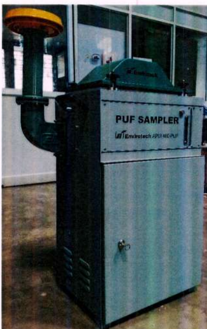
Fig 1: Ambient air PUF sampler
