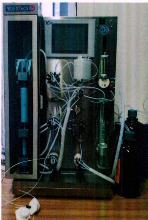
Fig 3: Automated Dioxin clean up system
